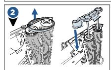
Replace Large Belt or Brush Rollers, as required, carefully reassembling the Rollers and Pivot Arm with attached rods and secure the Pivot Arm with the screw
