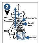
Remove the end cap first. Then, remove the only screw holding Pivot Arm, gently pull off arm to expose Roller ends
