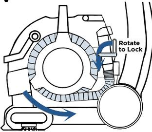
Make sure hose is wrapped. Rotate the latch to lock into place.
