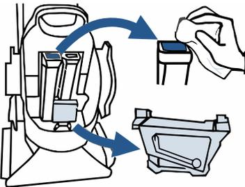
Clean the red filter and clear out any debris in the suction gate.
