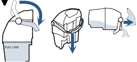
Rotate handle all the way over tank, remove top, pour out dirty water and rinse the tank.
