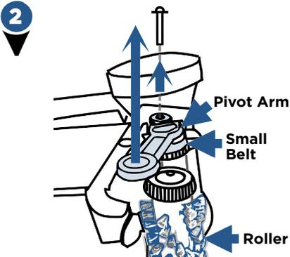
Remove the only screw holding pivot arm, gently pull off arm to expose ends of the brush rolls.
