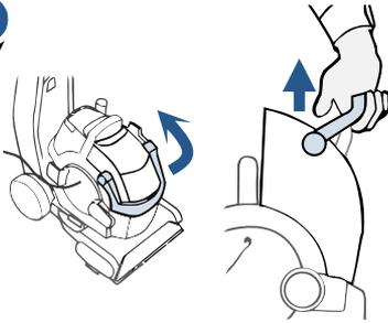
Swivel handle up and lift the dirty water tank away from the pod.
