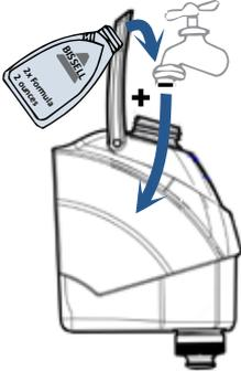
Remove cap, fill with hot tap water to the water line, and add 1.5 oz 2X formula to the 2X formula line.
