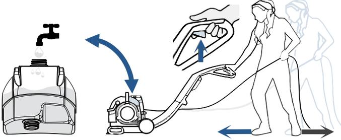
To clean machine before storing it, fill the Formula & Water Tank with hot tap water only, in order to flush out any residual formula
