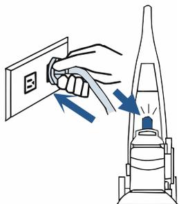
Plug into a properly grounded outlet. Indicator light turns on when unit is plugged in, power switch is pushed and pod is seated correctly.
