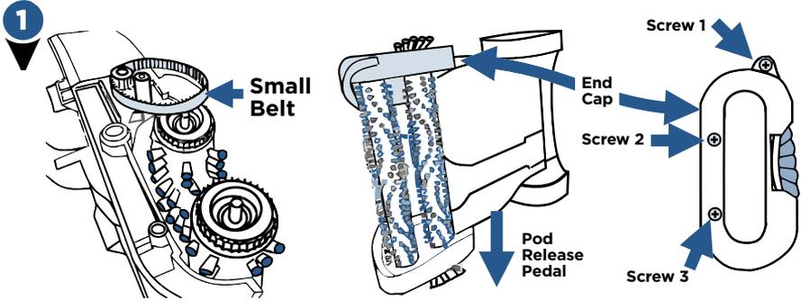
To replace **small belt**, flip the base unit to the side with the pod release pedal on the bottom.
