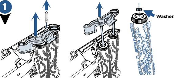
**IMPORTANT:** Do not lose the small washers held by a magnet at both ends of the brush roll.
