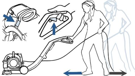
Press the trigger to apply solution.
