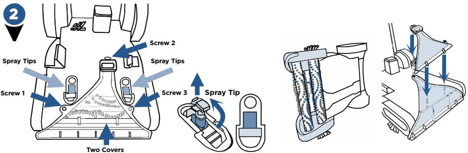
Separate the Pod from the base, remove the two Spray Tips, rinse at a faucet and replace
