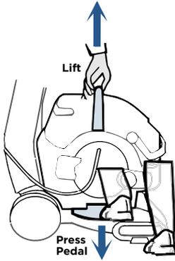
Separate pod from base to clean stairs or work on stained areas by stepping on pedal.
