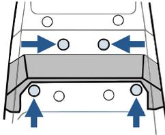
On the back, insert 4 screws in a slight upward angle.
